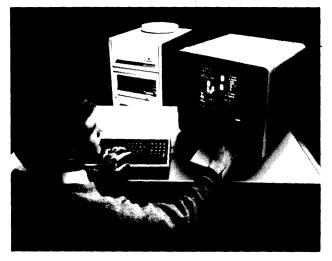
Digital Equipment Corporation's new VAX-11/730 32-bit minicomputer supports interactive graphics workstations using Digital's VS11 terminal for engineering design, educational, and commercial applications. The VAX-11/730 uses 64K-bit RAM chips for a maximum memory complement of five megabytes, and can be configured as a single cabinet system with prices beginning at less than \$50,000.
