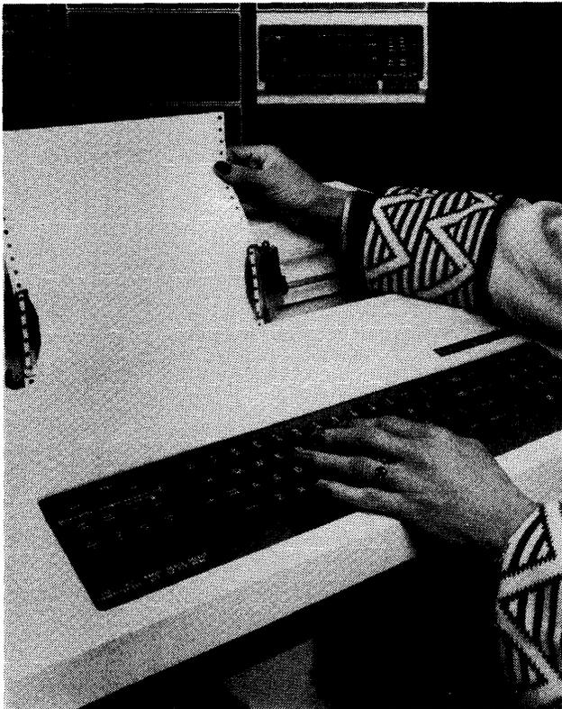
*The PDP-11/70 represents the high end of one of the most extensive minicomputer product lines in existence today. The PDP-11/70 is a high-performance machine with integral cache memory and high-speed 32-bit data paths. The system also has memory management, look-ahead, and internal memory expansion capability up to 4096K bytes.*
