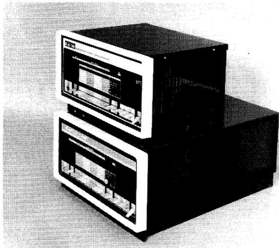
*The PDP-8/E on the bottom is the most powerful model in the long and extremely popular line of 12-bit minicomputers from DEC. The PDP-8/M perched above it is a lower-priced modular version for OEM customers.*
