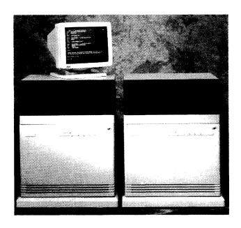
The new VAXft 3000 Model 310 features fully duplicated components in its fault-tolerant design.
