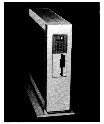
The MicroPDP-11/53 is typical of the downscaling that has occurred in the PDP-11 Family: the conventional minicomputers that used to comprise the product line have been repackaged as low-end multiuser microcomputers. The BA23 pedestal enclosure shown here is shared by MicroPDP-11, MicroVAX, and VAXstation systems.
