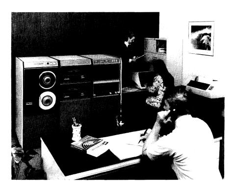
A typical single-user, interactive Datasystem 530 configuration is shown here. Based on DEC's powerful PDP-11/40, this system adapts well to small-business EDP environments. This particular configuration includes, from left to right, a 45-ips TU10D magnetic tape unit, 4.8 million bytes of storage provided by 2 RK05 disk drives, a PDP-11/40 central processor with 16,384 words of 1-microsecond main memory, a VT05 CRT display terminal, and a 132-position LS-11 dot matrix printer.
