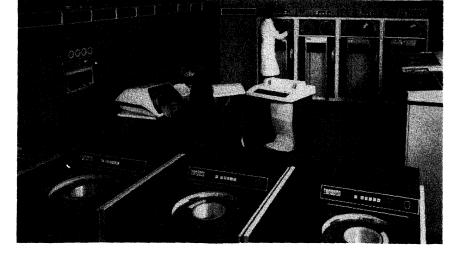
The DECsystem-1080, one of two new models introduced in October 1974, has twice the processing power of previous large-scale DEC computers and includes an extended instruction set for business data processing. It can be equipped with new large-capacity disk drives and highperformance magnetic tape drives.
