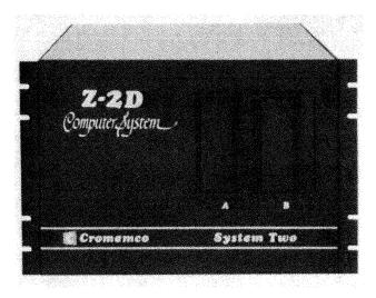
The System Two Disk Computer shown here is a complete, factoryassembled version of the Z-2D Disk computer. This system consists of two 5<sup>1</sup>/<sub>4</sub>-inch disk drives capable of storing a total of 184 KB, 64 KB RAM, and a printer interface. Price for the system as shown is \$3990. The Z-2 systems are all programmable in BASIC, FORTRAN IV, COBOL, or Assembler.
