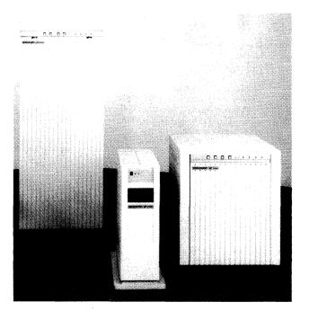
The XF/610, XF/400, and XF/600 superminis (shown left to right in the photo) make their debut as members of Concurrent's new Xelos Family (XF). The Xelos Family systems are based on modified Series 3200 processors and run AT&T's Unix System V, Release 2. The XF products support up to 16MB of memory, up to 2.4GB of disk storage, and a maximum of 64 communications ports.
