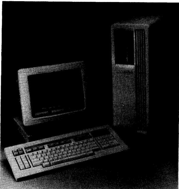
*Computer Consoles Incorporated's Power 5/32 runs under the Unix operating system and supports from 2MB to 4MB of main memory and from 85MB to 170MB of disk storage. The Power 5/32 uses the Motorola MC68010 microprocessor and can support up to 16 workstation users.*
