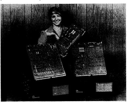
The LSI 4 family of processors includes the LSI 4/30, LSI 4/10, and LSI 4/90 (upper left to upper right). Packaged versions come in either an operator's console (lower left) or a programmer's console (lower right).
