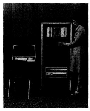
The top-of-the-line LSI 4/90 is shown with a programmer's console, floppy disk (top), medium-capacity disk unit (below), and CA's own CRT terminal. The 4/90 processor is priced at \$10,075 when configured with 64K words of 550-nanosecond memory, chassis, power supply, and operator's console.
