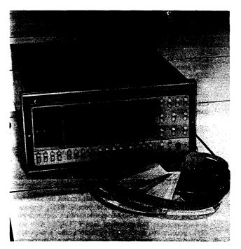
The 8-bit byte-oriented CIP/2200 Minicomputer has up to 32KB of 1.1 microsecond core main memory and up to 2K 16-bit words of 220 nanosecond control memory. The front panel has a matrix of indicator lights showing the status of key locations/ registers during processing. Often used in a computer numerical control environment (indicated by the paper tape/punched card input media), the CIP/2200 is supported by a general-purpose disk operating system.
