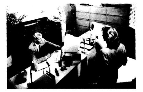
The new, compact Cyber 932 models are air-cooled superminis designed to work in a typical office environment. They run under the NOS/VE operating system and feature 8 to 128 megabytes of main memory and 6 to 12 I/O channels.
