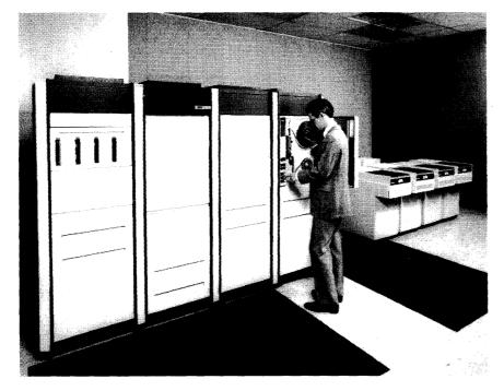
The BTI 8000 is a 32-bit multiprocessor packaged system designed to support up to 256 interactive users in a multilanguage, multifunction environment. The system, which is modular in configuration, can also support up to 24MB of main memory and 9GB of disk storage.
