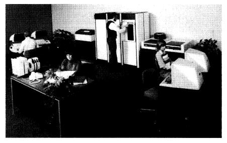
The BT1 8000 supports a number of peripheral devices and terminals. The BT1 8000 configuration shown here includes four terminals, two disk-pack drives, a reel-to-reel magnetic tape unit, and a line printer. This 32-bit system can support up to 200 interactive users in a multilanguage, multifunction environment.
