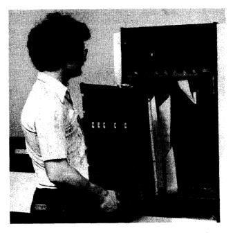
The hardware configuration of a BTI 8000 can be expanded by attaching additional "resource modules" to a high-speed bus. In the photo, a Computational Processing Unit is being plugged into the system cabinet. The bus circuitry is on the panel forming the back of the open area.
