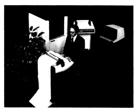
The BTI 5000 is shown with the optional Model 5620 (300 lpm) line printer to the right of the processor cabinet. The terminals shown are examples of units frequently used with the 5000. Terminals are not included in BTI's product offerings.
