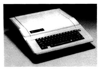
The Apple IIe was designed as a replacement for the Apple II computer. It provides 64K bytes of RAM expandable to 128K, an upper and lower case alphabet, and an extensive array of software.
