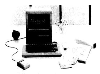
Equipped with Motorola's 16-/32-bit MC68000 microprocessor chip, the Macintosh includes 128K bytes of main memory, 64K bytes of ROM (which contains the operating system), an integral 9-inch screen and 3½-inch microdiskette drive, detached keyboard, mouse, learning manuals, and audio cassette. With the addition of a keyboard, mouse, manuals, and carrying case, the Macintosh weighs in at 23 lb. but its footprint is smaller than an 8½-inch by 11-inch sheet of paper.
