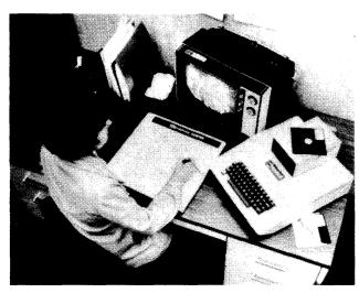
The Apple II, configured for fairly typical home use, includes a single diskette drive and a TV set for color graphics. Not as commonly used is the graphics tablet shown here, capable of producing highresolution, multi-colored drawings.
