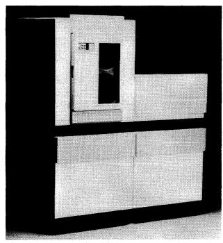
The 3B15, comprising Models 101, 201, 301, and 401, is the mid-range system in AT&T's 3B Computer family. The 3B15 supports up to 60 simultaneously active users. It runs under Release 2.1 of Unix System V, which provides demand paged memory management and record/file locking.
