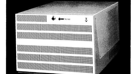
AT&T's 3B2/600 supermicrocomputer supports up to 64 active users and runs AT&T's UNIX System V operating system. The 3B2/600 is targeted for use as a departmental processor in large corporate environments.
