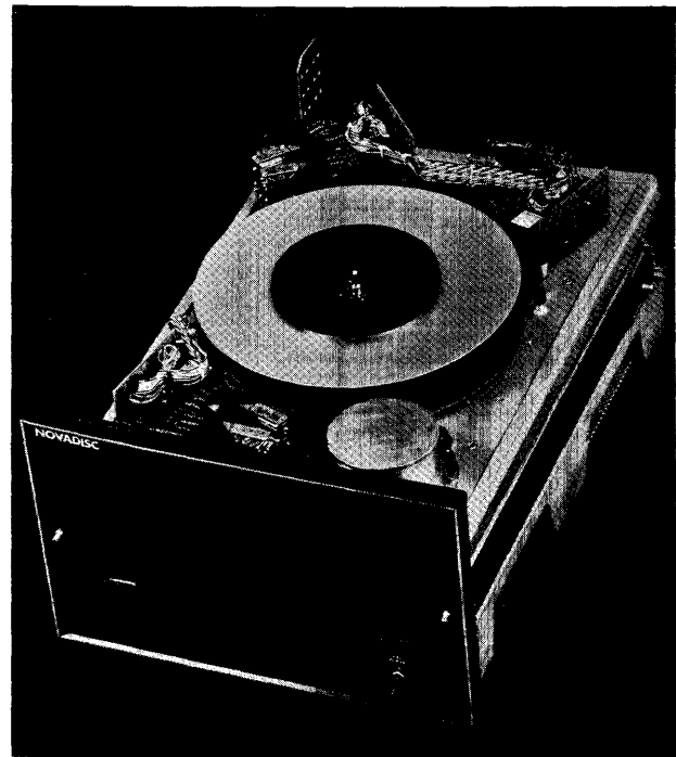
The more prosperous minicomputer manufacturers are beginning to enter the potentially lucrative field of peripheral building. This Novadisc unit from Data General features head mechanisms that swing out when the disk is stopped to prevent any contact of the heads with the disk surfaces.
