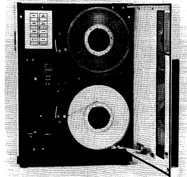
The Ampex TMZ tape unit features single-capstan drive (wheel at lower left), tension arms, and speeds up to 60,000 bytes per second. The tape path looks particularly complex; but, when loading, the tension arms move to the center so that threading in and around the guides is not necessary.
