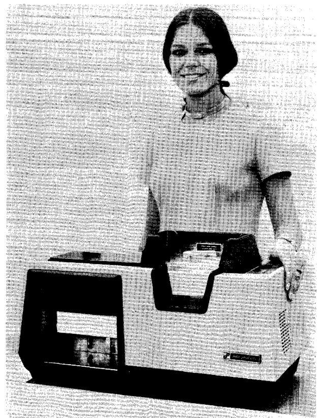
This neat model from Data Products (the 8330) shows the size of the current crop of tabletop card readers. It can read cards at over 300 cards per minute, which puts it at the low end of the line, and is one of the few units to use a picker knife mechanism.
