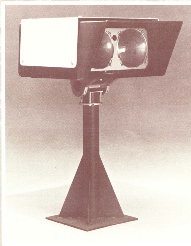
Datapoint's LightLink uses modulated non-coherent infrared light to transmit information across short distances.
