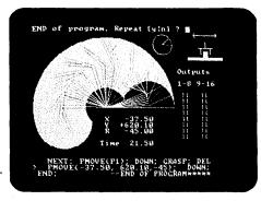
Figure 2. This display from the AML/Entry Application Simulator is used to check the logic and efficiency of an AML/Entry program, display the robotic arm manipulation (from above), and provide timing estimates.
