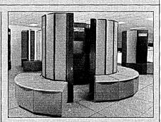
memory, respectively. On the 4 millionword system, memory is arranged in 32 interleaved banks, and on the 1 and 2 million-word systems, it is arranged in 16 banks. Memory bandwidth is four times that of the Cray-1.
