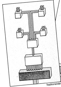
Model 6641 Line Expanders direct data from an IS/3M 6632 Multiplexer attached to the IBM 3274 Controller to one, two, three, or four IS/3M6600 Mutliplexers that can be arranged in a variety of network
