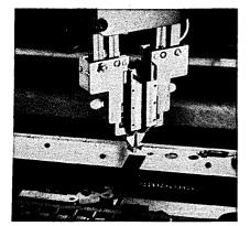
Figure 4. In the automatic assembly of ype chains for an IBM high-speed printer-one of the many examples of BM robotic systems at work within the company-an AML program is used to consult a data base to determine the correct sequence of type slugs. This upplication makes extensive use of sensing and programmed error recovery to ensure high reliability.
