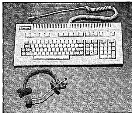
utility program. The vendor says the unit has a speech recognition accuracy of 98% or better. Words from any language can be used, since the system is trained by the operator. The intelligent keyboard recognizes discrete words and phrases lasting no longer than 1/4 seconds, with a brief pause of a quarter of
