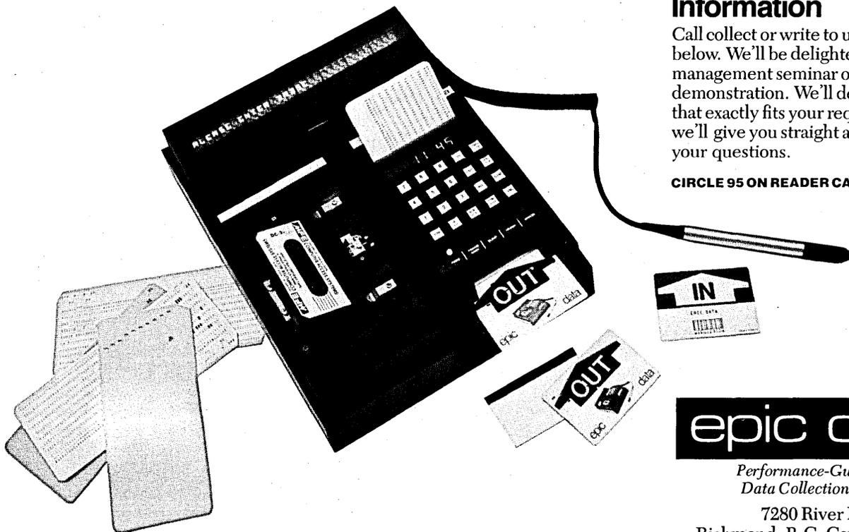
*Epic terminals accept data from punched or magnetic stripe badges, punched cards, barcodes or through the keyboard. They hold the input data in memory or on cassette, or pass it along to an Epic Data control unit, the host computer or a peripheral device. Each of these functions is available in a separate Epic terminal or in your choice of combinations.*
