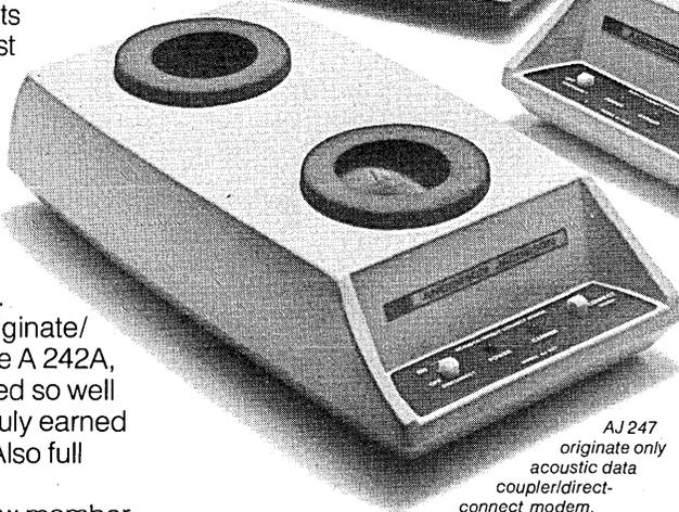
AJ 247 originate only acoustic data coupler/direct-connect modem.
