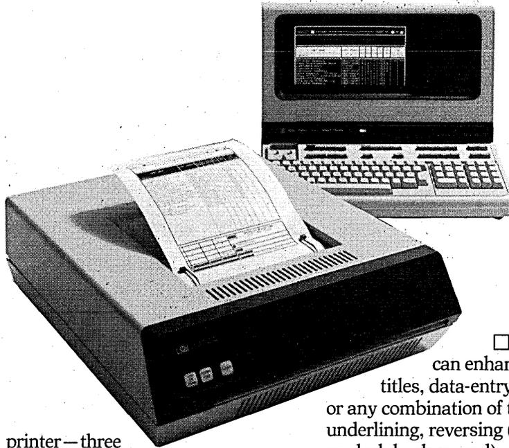
printer — three are dedicated to two 128-character ASCII sets (fixed and proportional spacing) and 25 Roman Extension sets, and the remaining three ROMs provide three of four optional character sets.
