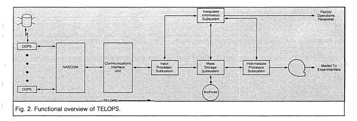
(GSFC) and IBM, and features a mass storage system that combines the data capacity of a large tape library with the access speed of on-line disk storage, and includes a communications input unit that accepts input rates up to 2.688 million bps with simultaneous outputs to the remote stations for retransmissiion requests at up to 1.344 million bps.
