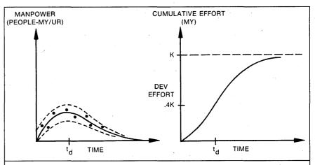
Fig. 2. The curves defined by this equation, originally applied by Lord Rayleigh to describe other scientific phenomena, have been found to fit reasonably well the manpower pattern of software development, at least within the "noise" of the data points (lefthand curve).
