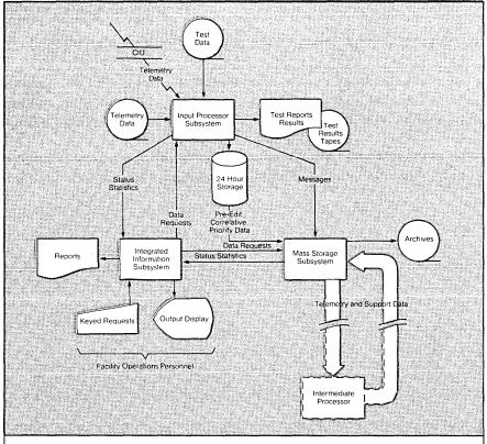
Fig. 5. TELOPS operational data flow.
