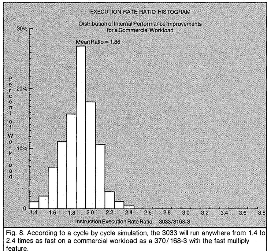
Fig. 8. According to a cycle by cycle simulation, the 3033 will run anywhere from 1.4 to 2.4 times as fast on a commercial workload as a 370/168-3 with the fast multiply feature.
