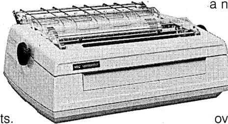
instant. An operator-controlled "impact scaling" switch modifies hammer energy to light, medium or heavy impact, depending on the form type and thickness.
