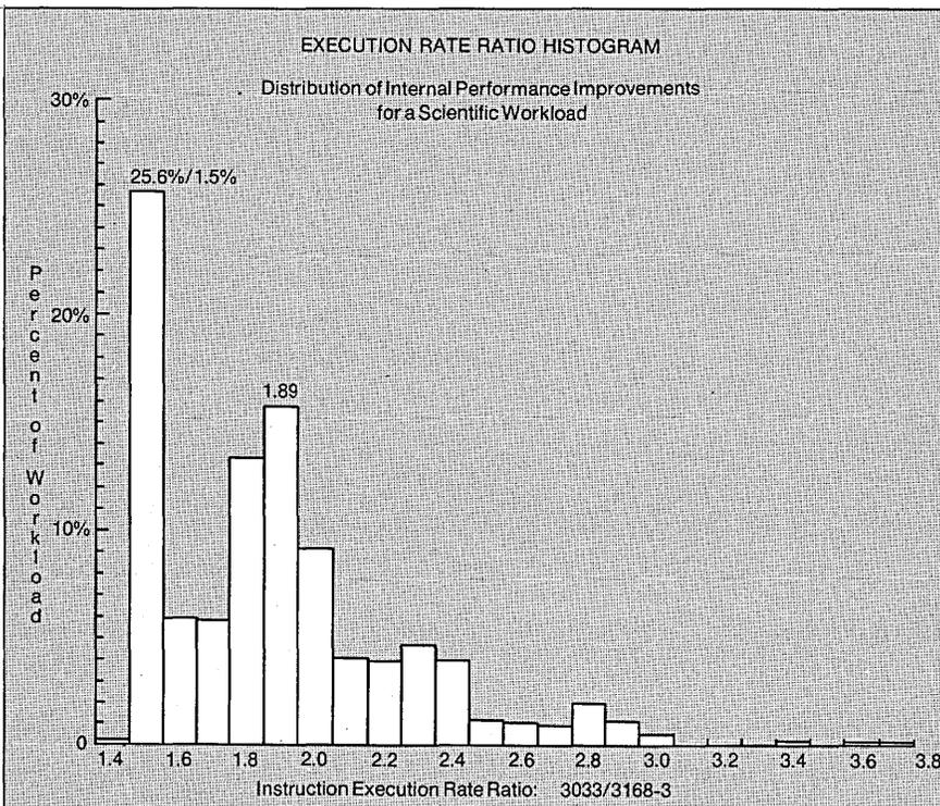
Fig. 9. On scientific workloads, the 3033 again appears to be just under 1.9 times as fast as a 168-3 with the high speed multiply feature. Some optimized FORTRAN execution steps are very well suited to the 168, however, and the 33 can manage only 1.5 times the instruction execution rate for those.
