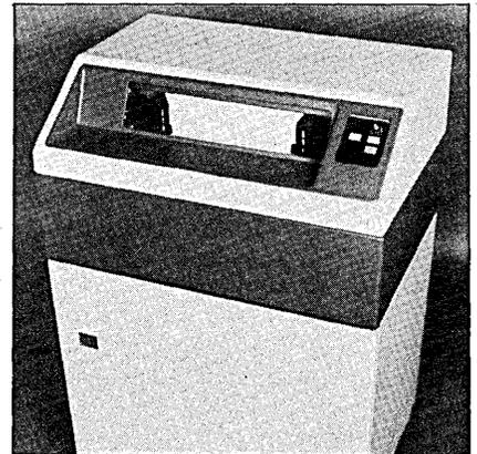
swing-out yoke and in-line paper tractors simplify forms loading, and 69 interchangeable type bands, covering 22 languages, are available. A 300 lpm model sells for \$5,995, a 600 lpm model is \$8,995, and a 900 lpm unit goes for \$12,995.
