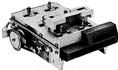
Here is a unique reader for use in the wagering market: it can process two completely different sized betting tickets. Tickets can be different widths and/or different lengths. Once read, they are returned to the operator. The mechanism can be fitted with the conventional mark sense head or with PDI's new broad spectrum sense head—whichever the application requires.
