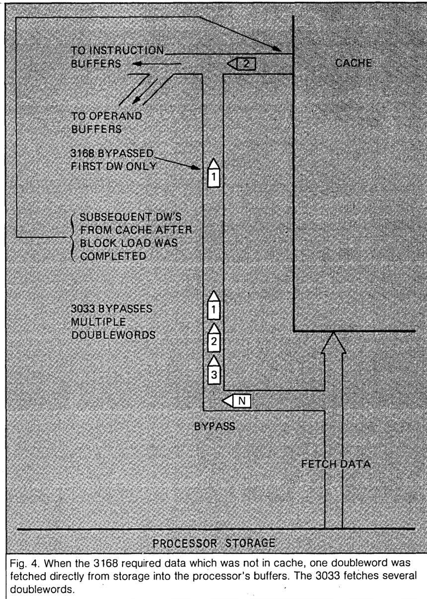
Fig. 4. When the 3168 required data which was not in cache, one doubleword was fetched directly from storage into the processor's buffers. The 3033 fetches several doublewords.
