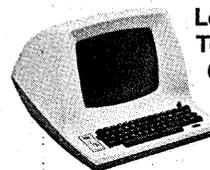
**Lear Siegler ADM-3A Data Entry Display Terminal** 12" diagonal, 24-line screen. 64 ASCII characters. Full or half duplex operating modes, switch selectable, baud rates from 75 to 19,200. RS232C interface, 20mA current loop.
