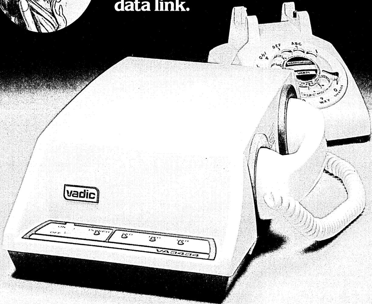
Racal-Vadic is in full production on an acoustic coupler that operates at 1200 bits per second, full duplex. Thousands are already installed and operational.
