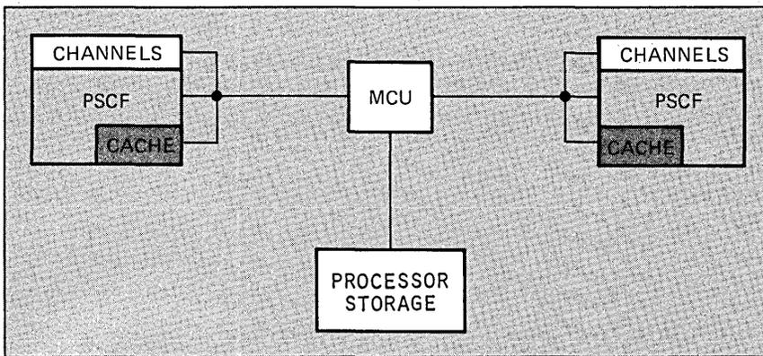
Fig. 5. Both the Multiprocessor (MP) and Attached Processor (AP) configurations employ a Model 3038 Multiprocessor Communications Unit. The MCU lashes processors and main memory together with 8-byte wide data paths.
