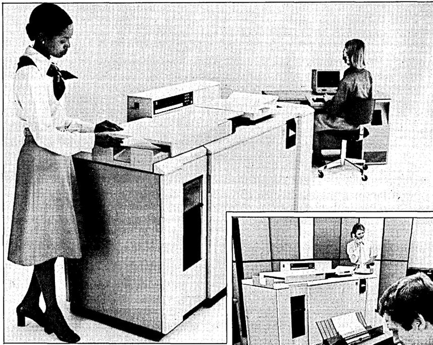
IBM 6670: The information distributor uses a laser printer to provide original quality printing for each page either through communications lines or magnetic cards. It can be used in conjunction with the IBM Mag Card II typewriter (at right). Laser technology enables it to print up to four separate type styles on a single page in any sequence.
