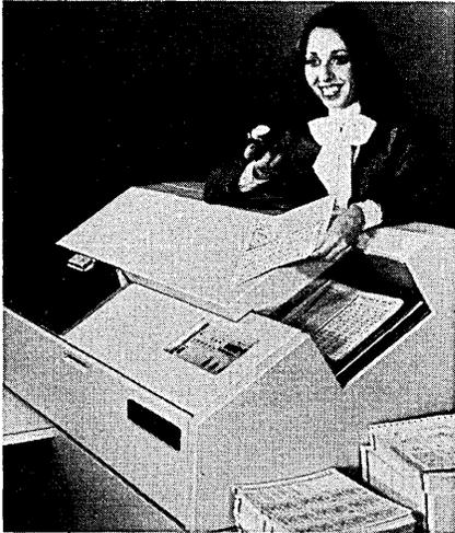
cpu as a 2780 or 3741; off-line it can prepare seven or nine track mag tapes at 800bpi or 1600bpi. The unit can handle forms ranging in size from 3½ X 7½ inches to 8½ X 12 inches. A "sheet compiler" is used to describe forms to the scanner. It defines fields to be scanned, output formats, edit checking, and if desired for grading, right answers and a grading formula. Scanner lease prices start at \$975 per month. NATIONAL COMPUTER SYSTEMS, Minneapolis, Minn.
