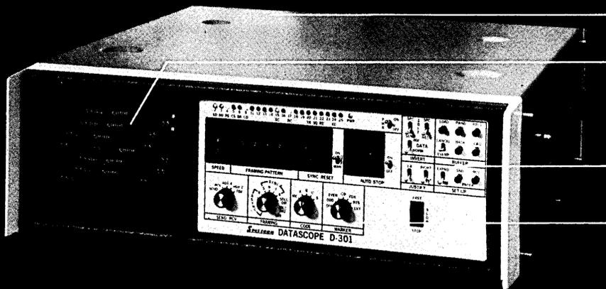
The fully microprocessor-based D-301 is designed for portability. It's a 5 1/2" high x 16" wide x 17" deep, brief case size, and weighs only 25 lbs. It has a built-in ease and simplicity of operation, as do all DATASCOPEs.
