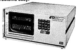
The Hawk 4000. It's IDS's new Data Trap with a microprocessor that lets you diagnose data communications problems quickly. The Hawk is interactive. It can monitor, transmit, and receive data between a modem and terminal on a big 9", 512 character screen. And, 2000 characters can be trapped and stored for later recall and study.
