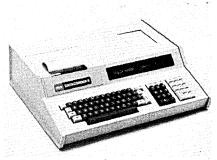
1pm printer, full ascii keyboard, and an Rs232 interface. Peripherals and options include a choice of line printers, 9-track mag tape, an additional cassette drive, external peripheral ports (serial or parallel), and memory expansion to 64kB.
