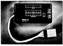
provides single step, hardware breakpoint, and oscilloscope trigger capabilities. LED's display the status of the data and address lines. The MSA-8 sells for \$249. COMPUTER SYSTEMS DYNAMICS, Salt Lake City, Utah.
