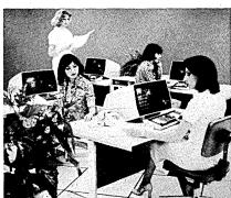
We learned, for example, that a large display screen makes an operator station easy to use. A 15-inch, non-glare CRT is standard on all Series 21 systems. We learned that some record formats fit well on a 480-character screen while others require 1920-character capacities. Series 21 offers both, under program control, and displays 7x9 dot matrix characters in green against a green background — a combination we've learned is easy on the eyes.
