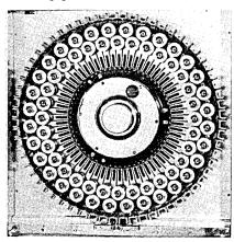
tually a 3.1MB mass storage device. The ECM-64 FACIT contained 64 randomly selectable tape cartridges on its carousel.
