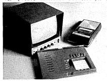
\$275 computer on a card with an eight-bit microprocessor, operating system in 512 bytes of ROM, 2KB of
