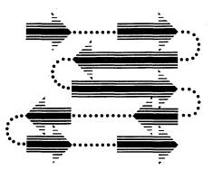
The HP 2631/2635 choose the most efficient direction (left-to-right or right-to-left) for the print head to move. Smart, bi-directional printing can increase throughput as much as 50%.
