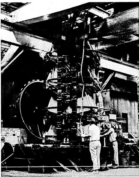
This heat-treating machine, called an autoclave, bonds auto windshield laminations. DL/1 helps Libbey-Owens-Ford control production to meet demand for a fast-growing list of part numbers.
