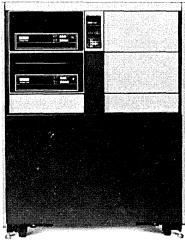
the ability to run even when parts of the CPU are down. And if you do your own maintenance, the optional Diagnostic Control Store module can troubleshoot to the board level in seconds.
