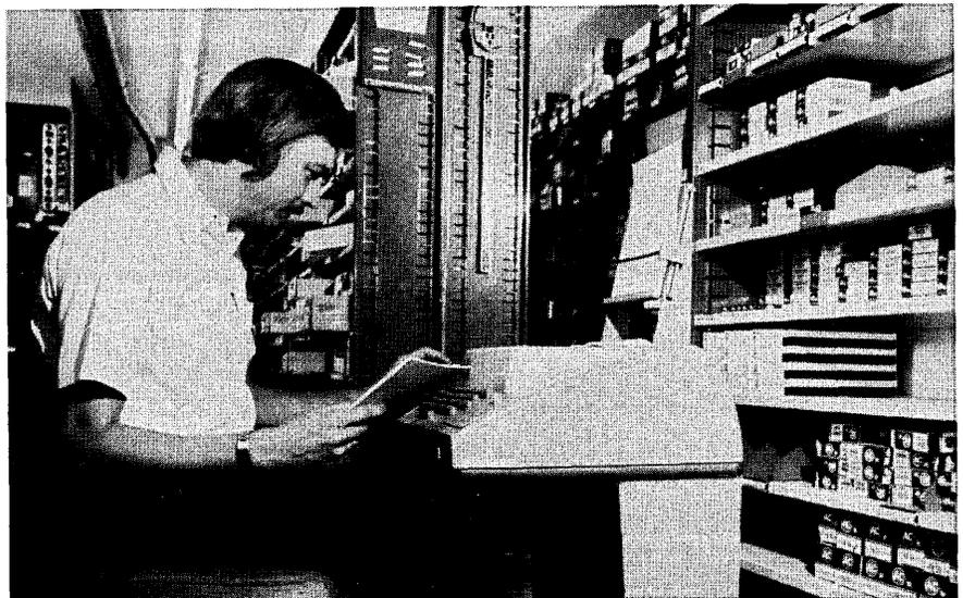
Terminals in 4,500 GM parts departments are the base of a communications hierarchy which includes 29 cpu's at parts warehouses, at least eight more at four regional centers, and one at the GM Parts Div. headquarters in Flint.
