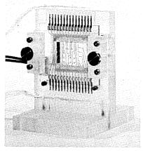
The heart of the memory is a two-inch square section of transparent recording material capable of storing 409,600 bits of dynamic storage, or 13 megabits of read-only storage.
