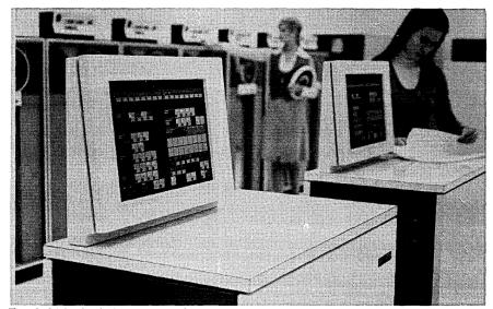
The 3704 is the baby brother of the 3705 announced last year. Both the 3704 and the 3705 can now be used as remote communications concentrators. Both products are programmable only via 370 systems.
