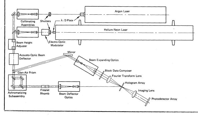
(reference) beam are then both flashed on the recording material. The top layer heats to approximately 70°C, whereupon it softens. The positive charges atop the thermoplastic material tend to push it toward the negatively charged lower material, deforming the top layer into the Fourier transform of the
