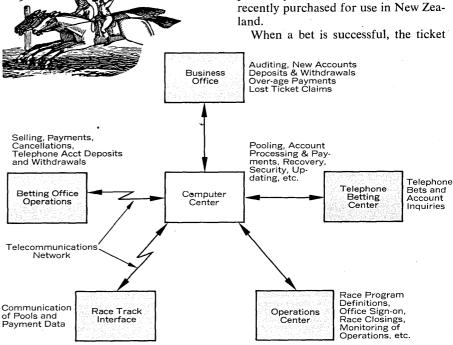
Fig. 1. Schema of the principal system components
