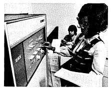
number of language processors are available, including ANSI FORTRAN IV, extended SYMBOL, RPG, SORT, DEBUG, and a scientific subroutine library. A typical 530 would be a system with a line printer, disc storage unit, card reader, and console. This configuration, available in the third quarter, is priced at \$62,900 and can also be leased. XEROX CORP., El Segundo, Calif.
