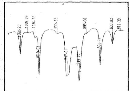
Plot of infrared spectrum with peaks found by program and labeled.
