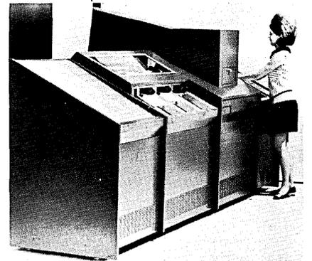
printed character vocabulary is less extensive; the machine recognizes the numerals 0-9, the letters C, S, T, X, and Z, and plus and minus signs. With these characters, users can print very much as they always do, because the machine defines characters by features such as curved lines, sharp corners and line intersections.
