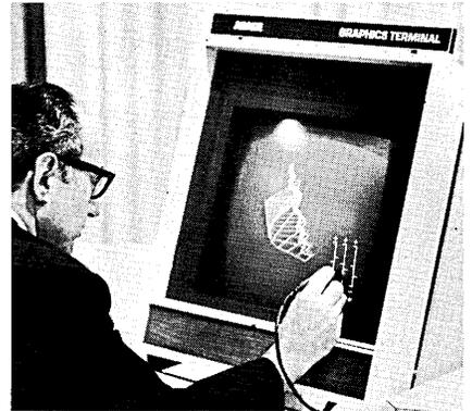
of programs. The user has access to the capabilities of the terminal via programs written on the computer. Image files are transmitted to the AGT for processing and display. Control files are used to activate the keyboard and the light pen, and to sample the function switches and any other interactive controls. The editor, assembler, and debugger are provided for support and maintenance of the communications and formatting routines.
