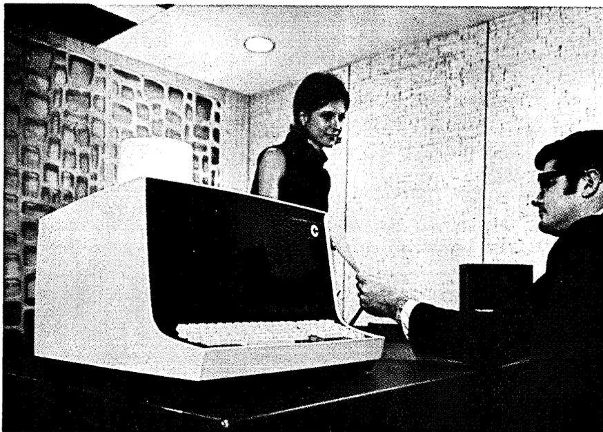
take in a complex problem situation at a single glance, make revisions, corrections or deletions for any combination of lines or characters via the keyboard; you can debug on-line; you can in effect make the computer an immediate and powerful extension of your own thought processes.
