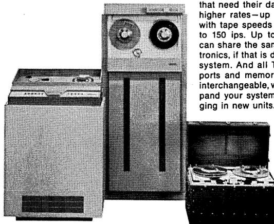
TM-11 and TM-12 transports/memories are designed for systems that need their data transferred at higher rates—up to 120,000 cps—with tape speeds ranging from 75 to 150 ips. Up to four transports can share the same memory electronics, if that is desirable for your system. And all TM-series transports and memories are interface interchangeable, which lets you expand your system simply by plugging in new units.
