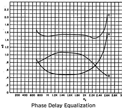
The newly designed Model 25400 Adjustable Delay Equalizer is totally compatible with all RFL data sets as well as all other data transmission facilities. This variable system provides precise equalization of communication paths with respect to either phase or amplitude, or both, which is essential to high-speed data transmission. Resultant flat response
