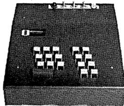
**Model 117, Encoding Keyboard . . .** 18 key . . . converts key depressions into coded (8 level) arrays of switch closures designed to interface with tape punches, printers, plotters, computers or other automatic machinery. Any code configuration can be supplied. Keys can be mechanically or electrically interlocked. **Price: \$435.00**
