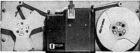
**Model 110, Paper Tape Punch . . .** punches standard 5 to 8 channel paper tape asynchronously at speeds up to 30 CPS. Powered by continuously running induction motor. Error detection achieved by parity checking switches. Tape can be back-spaced. 7"x 19" panel, 24 or 48 VDC. **Price: \$599.00**
