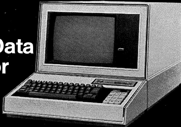
RCA's 70/752 Video Data Terminal is a CRT display with separable keyboard that provides direct communication with a computer for data entry and retrieval. This third-generation unit has a transmission speed of 120 cps and will display up to 1080 characters at once (20 lines of 54 characters each). Off-line editing permits data to be changed or inserted anywhere in the message. Up to 26 terminals can sequentially communicate with the computer over a single leased telephone line.
