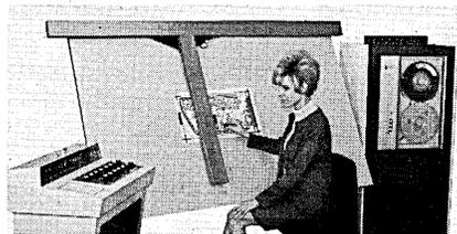
ruled glass scale. Measurements are taken from maps, drawings, etc., and are recorded in computer compatible formats onto punched cards, paper or
