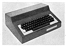
photo-resistors produces changes in their individual resistances. These ohmic changes are available as direct outputs or may be converted by amplifiers to corresponding voltage level changes. The amplifiers have low output impedances and may be connected to other data system devices. INVAC CORP., Waltham, Mass. For information:
