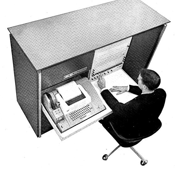
Our SEL-840A is the only computer in its class that offers an independent, concurrent, extended arithmetic unit (EAU) with a complete set of 22 additional hardware commands. The EAU performs 11 digit floating-point calculations as well as single and double-precision fixed-point calculations.
