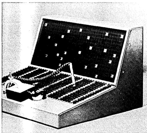
DATA-PANEL, with 540 lamp display is used in Module Test Device at Litton Data Systems Division.
