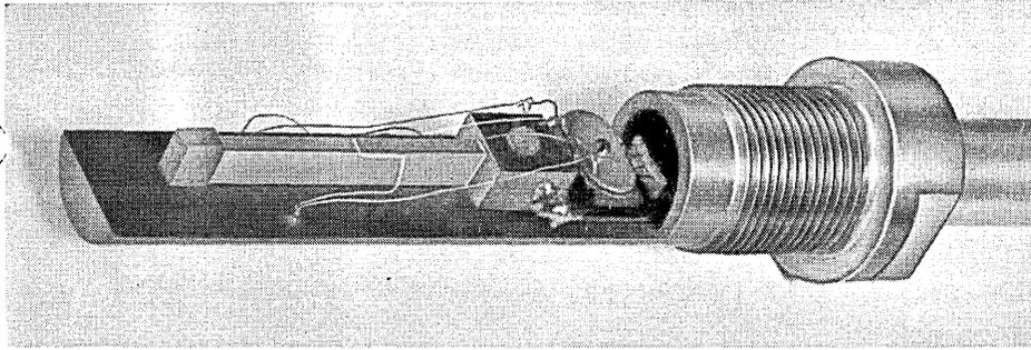
An elegant, but tiny refrigerator, utilizing the Nernst-Ettingshausen effect, has been demonstrated in the Solid State Physics Laboratories at Lockheed Missiles & Space Company. This type of cooling is applicable below 200° Kelvin, where thermoelectric cooling is no longer efficient. It shows particular promise for space application because of the reliability inherent in its all-solid state construction.
