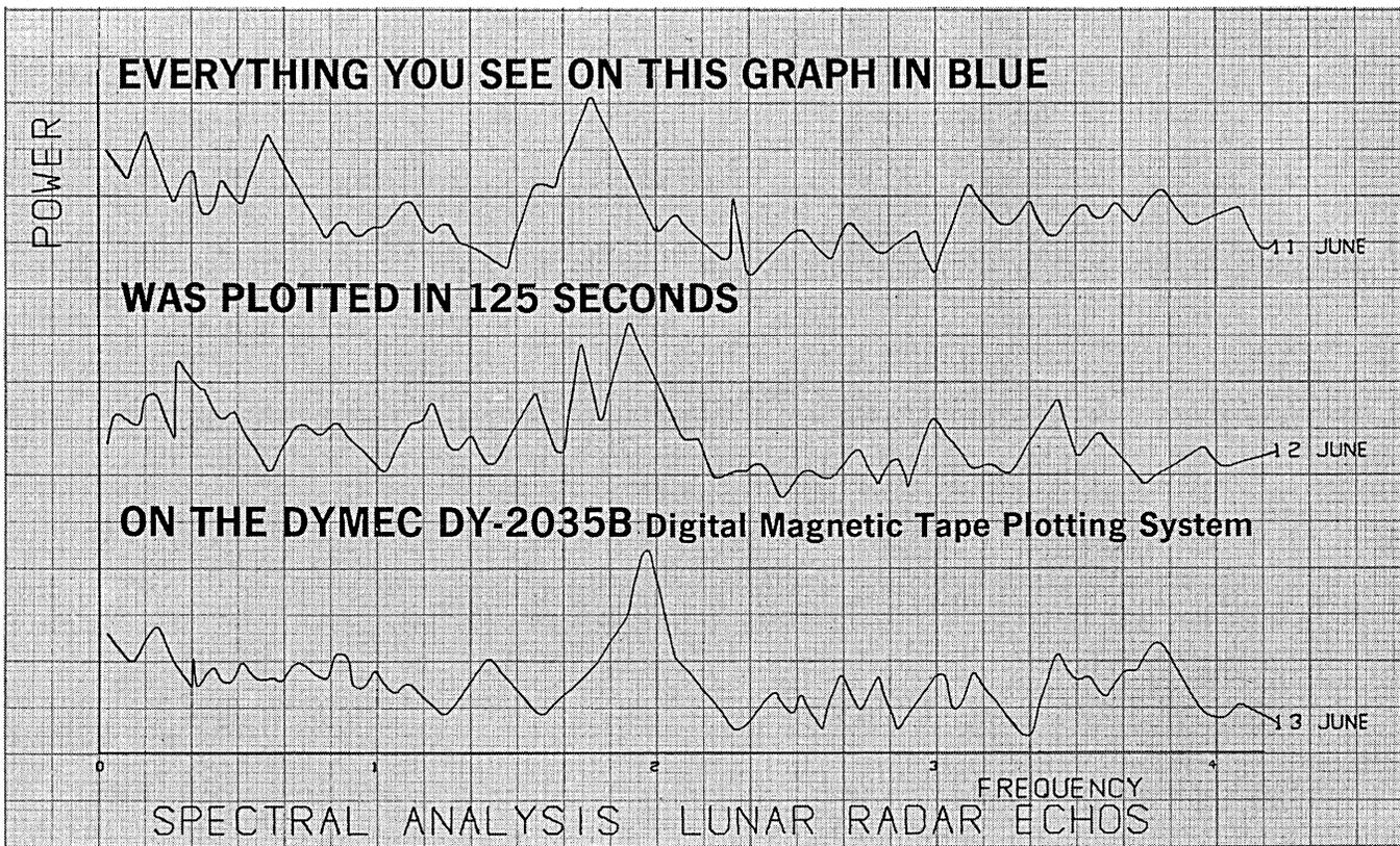
Fast plotting of digital computer data stored on magnetic tape is yours with the DY-2035B System which provides an average plotting speed of 4 inches per second, with slewing as fast as 20 inches per second.
