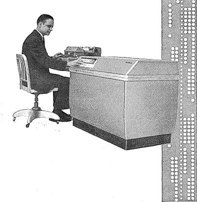
Remarkably simplified command structure and controls require only minimum computer experience. Front panel oscilloscope for concise display.
