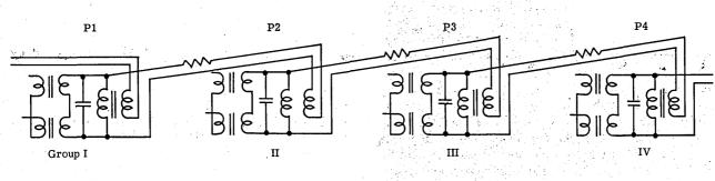
Figure 3. A shift register with parametrons
