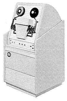
width tape, from five to eight level code. Plastic reels are available in two sizes, for tapes of 350 or 700 feet (40,000 or 80,000 characters). Features include automatic rewind and end-of-tape sensing, true straight-line loading and drift-free design. The photoreader is available as a component for mounting in any standard 19" cabinetry. For information write ELECTRODATA DIVISION, Burroughs Corporation, 450 Sierra-Madre Villa, Pasadena, Calif. Or use card. Circle 173 on Reader Service Card.
