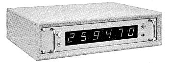
erates in response to a 1-2-2-4 binary code supplied by the manufacturer's counting instrument or some other source. The in-line indication does not change while the counter is actively scaling, but changes only at the end of a counting interval, at which time it displays the new total. Maximum display rate is 15 presentations per second. (Beckman/Berkeley Division, Beckman Instruments, Inc., 2200 Wright Avenue, Richmond 3, California.)
