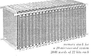
Because TELEMETER MAGNETICS manufactures the memory system complete from core production through array wiring to finished units ... and because TELEMETER MAGNETICS tests each phase of production thoroughly  $\ldots$  you can be that much surer when you specify memory systems designed and engineered by TMI.
