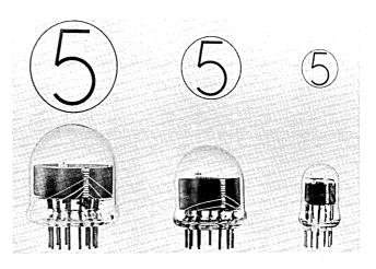
at a 50 KC rate. There are four basic types available: BD-200-S miniature, 6844-A standard, 7153 super, and BD-307 jumbo. (Electronic Tube Division, Burroughs Corporation, Plainfield, New Jersey.)
