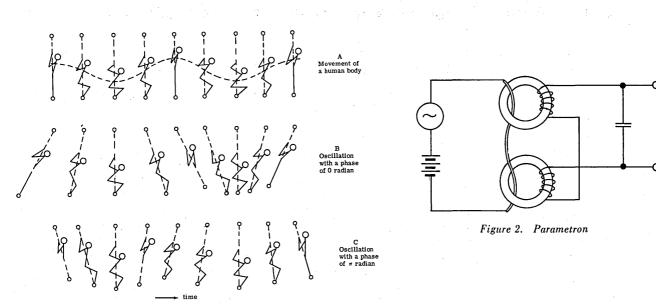
Figure 1. Parametron principle in a swing.
