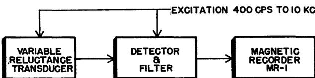
Fig. 6. Typical variable reluctance transducer circuit.
