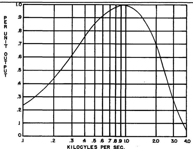
Fig. 7. MR-1 system frequency response with 1-mil gap heads (direct recording only).
