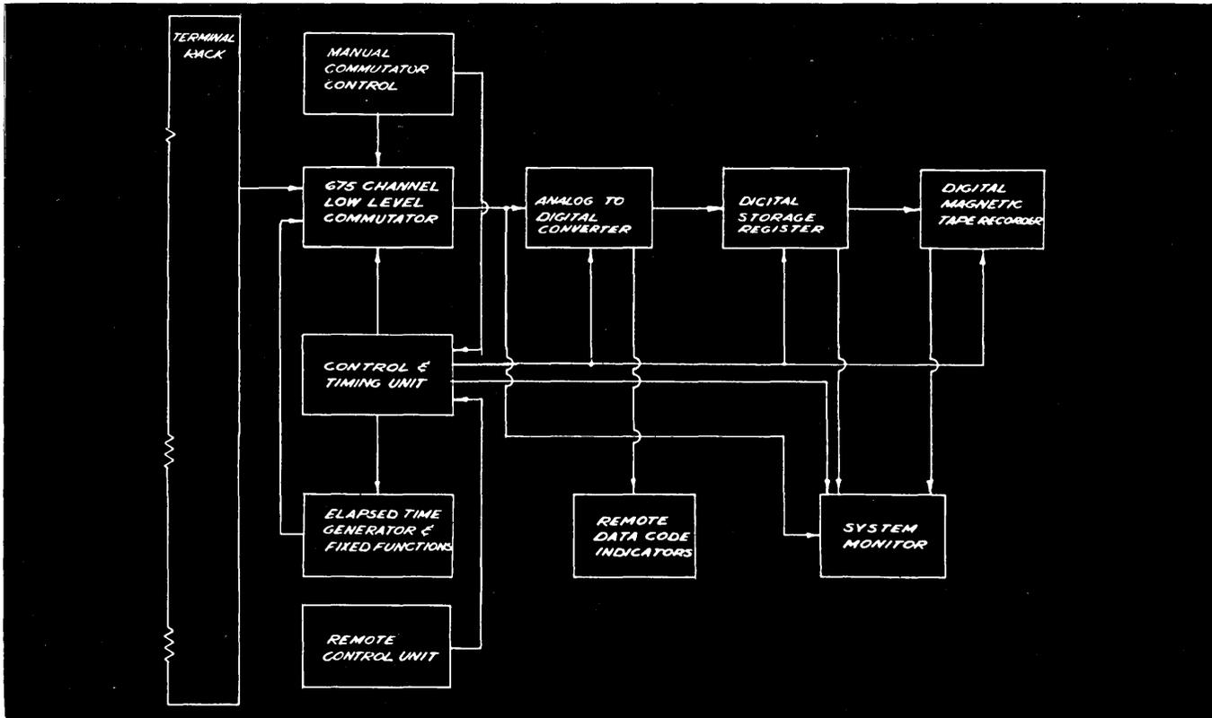
Figure 3. Block diagram of digital system.
