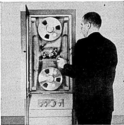
AMPEx CORP., 934 Charter St., Redwood City, Calif., has announced a new digital computer input/output system that offers rates as high as 90,000 6-bit characters per second. Known as the Ampex Digital Tape System, it consists of 4 interdependent items: tape handler, read/write heads, electronics, and a special magnetic tape.
