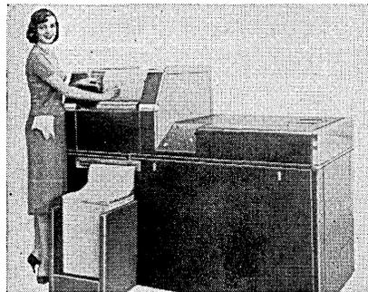
POTTER INSTRUMENT Co., INC., Sunnyside Blvd., Plainview, L. I., N. Y., has announced a new alphanumeric printer, the Magnityper, that combines such mechanical and circuit features as integral housing of the mechanical printing assembly with the electronic storage and comparator system, input adaptability to any source of digital data, and solid state devices, both transistors and magnistors, with modular-type construction.
