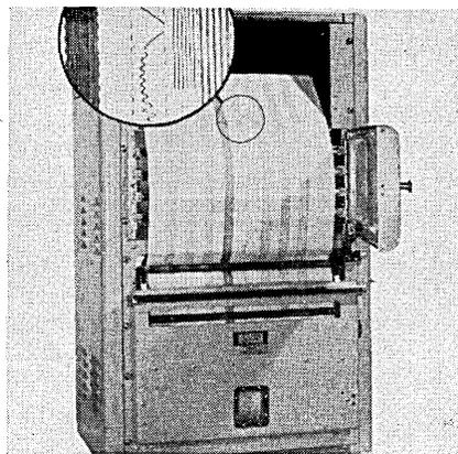
HOGAN LABORATORIES, INC., 155 Perry St., New York City 14, has announced a new 450-trace quick-look direct instrument recorder for use with digital data reduction, telemetry output recording, spectrum analysis work, and general off-on event displays.
