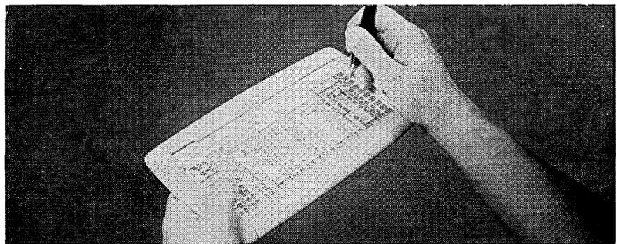
Port-A-Punch for on-the-spot recording of info in punched hole form.
