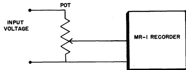
Fig. 2. Typical potentiometer transducer connection.
