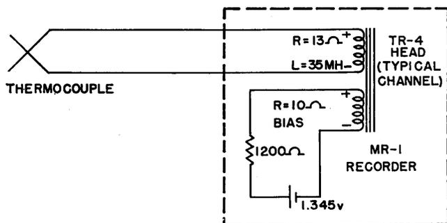
Fig. 3. Typical thermocouple circuit.
