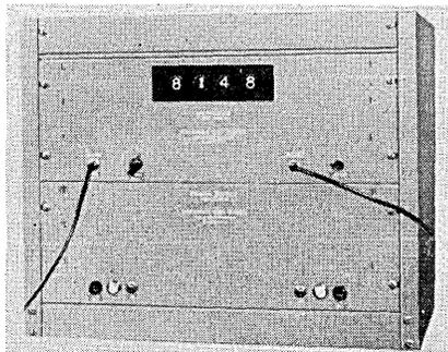
BURROUGHS CORP., Electronic Tube Div., Plainfield, N. J., has announced a 4-decade instrument, the Optimeter (Occurrences per time interval meter), which counts, samples, stores, and provides a working output without the need
