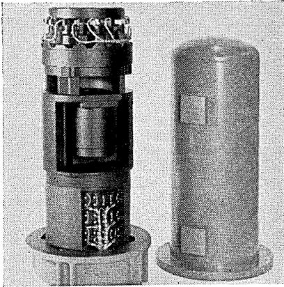
CONSOLIDATED ELECTRODYNAMICS CORP., Transducer Div., 300 N. Sierra Madre Villa, Pasadena, Calif., has announced a new device for PDM commutating and coding. Termed the Type 40-101 Plexicoder, the instrument commutates signals from up to 90 transducers at 112.5 samples per second and converts them into duration-modulated pulses suitable for telemetering or magnetic tape recording.
