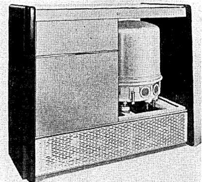
LABORATORY for ELECTRONICS, INC., 141 Malden St., Boston 18, Mass., has announced a high-density magnetic file drum, the HD, that stores 1040 bits/in., has 320 tracks (20 tracks are spares), and stores a total of 15 million bits. Access time to stored data is 180 milliseconds (average). The unit consists of a file drum (15" in dia. by 14" tall), drive and lubrication systems, a 3 by 10 by 10 track-selection mercury relay matrix, a linear read-out preamplifier, and a final writing amplifier.
