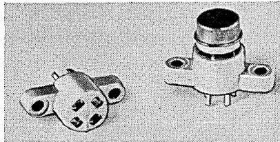
GRAYHILL, INC., 561 Hillgrove Ave., LaGrange, Ill., has announced a new socket for use with the new 3 and 4 Pin Jetec 30 transistors. The socket body is molded from mica-filled phenolic per MIL-M-14, Type MFE. The beryllium copper contacts are wrap-around style, silver-plated, and gold-flashed for contact and corrosion resistance.
