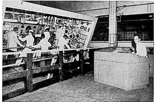
Signals are fed to oscillograph through amplifiers from ancillary computers and from analog computer.
