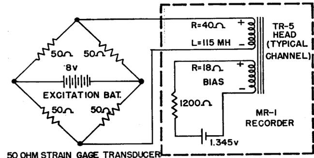
Fig. 4. Typical strain gage circuit.
