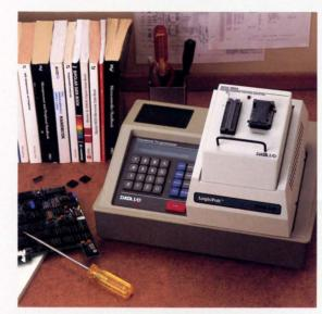
Equipped with the LogicPak™, Data I/O's 29B, 29A, or 19 mainframe becomes the sophisticated Programmable Logic Development System (PLDS) for designing, programming and testing virtually every programmable logic device
