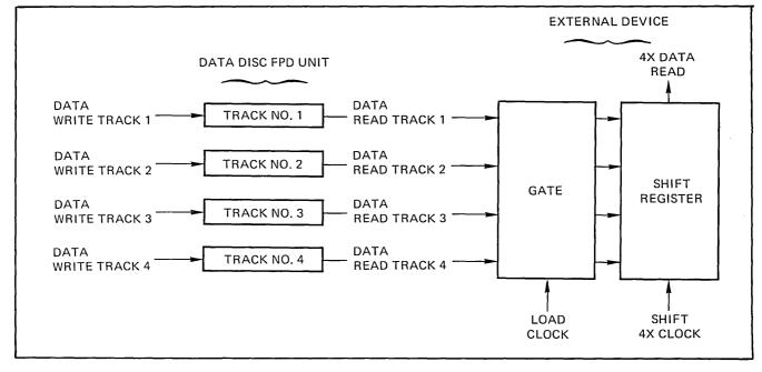
Figure 2-3 Four Tracks Read in Parallel and Serialized at a 4X Rate
