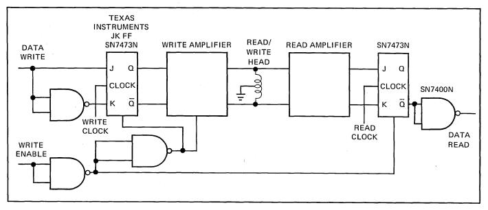
Figure 2-1 Read/Write Module
