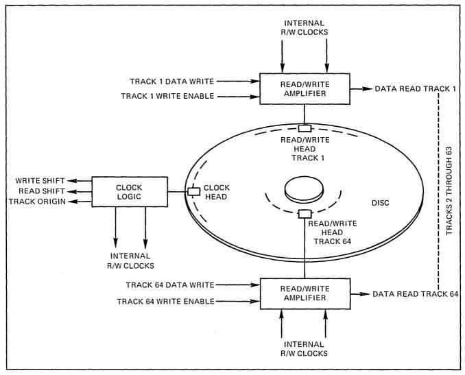
Figure 2-2 FPD Disc Memory System Block Diagram
