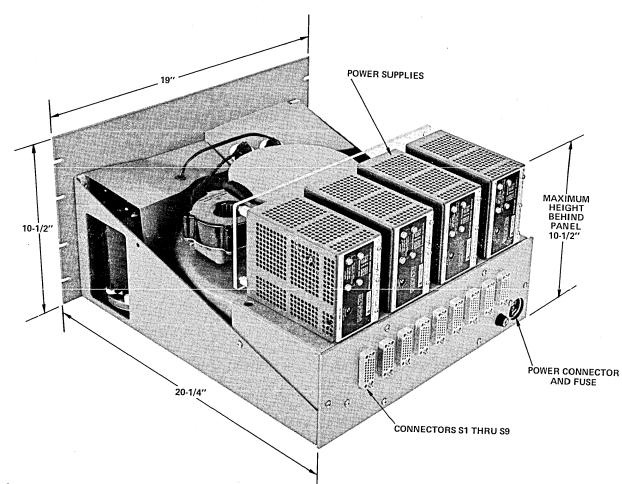
Figure 2-5 FPD Disc Memory System, Rear View
