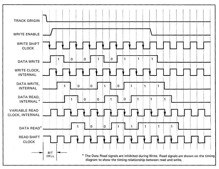
Figure 3-2 Timing Diagram
