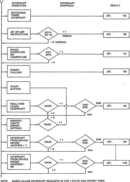
NOTE MASKS ALLOW INTERRUPT REQUESTS IN THE 1 STATE AND INHIBIT THEM IN THE 0 STATE. ALL INTERRUPTS PUT THE CPU IN THE EXTENDED ADDRESSING MODE AND SET INH/ENB TO INH PREVENTING ANOTHER CONTOLLED INTERRUPT UNTIL THE FIRST IS HANDLED.
