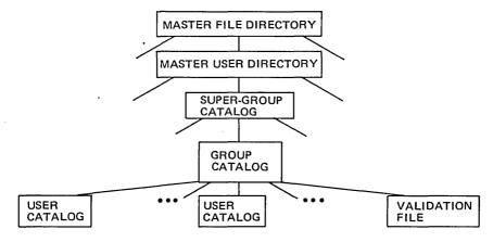
Fig. 6.5 - User Catalogs and Validation Files in the DTSS File Structure.
