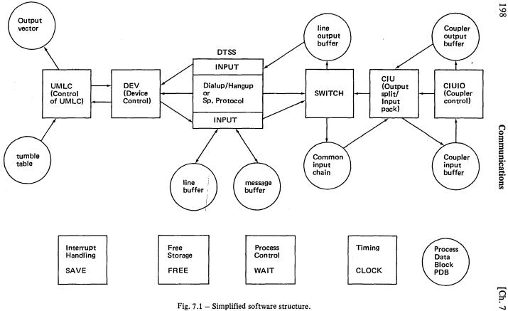
Fig. 7.1 – Simplified software structure.
