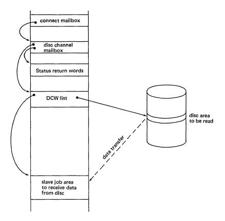
Fig. 5.11 – Pointers for a disc read.
