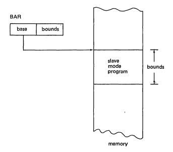
Fig. 2.3 - Base address register.
