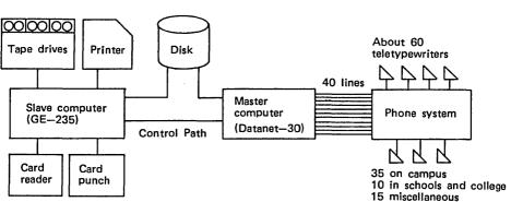
Fig. 1.1 - Hardware and communications for the first DTSS.
