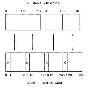
Fig. 2.4 - 716 to level 66 mapping.
