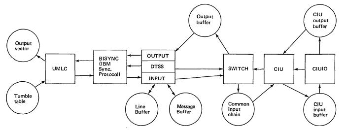
Fig. 7.9 – Binary synchronous protocol routines.
