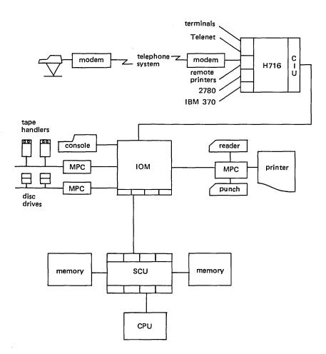
Fig. 2.1 - Honeywell series 60 level 66 architecture.
