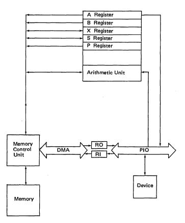
Fig. 7.3 – Device connections.
