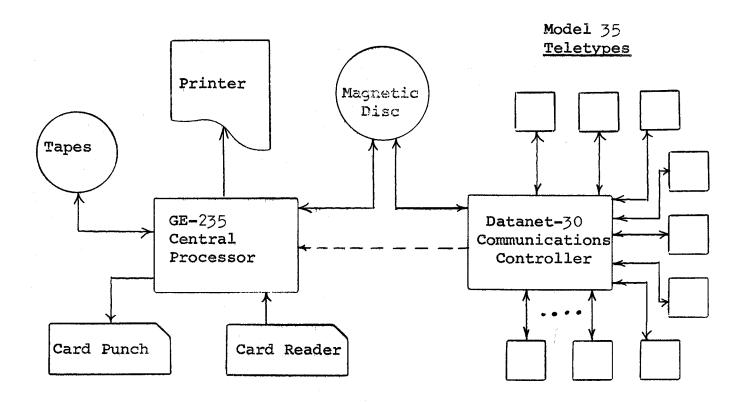
Schematic Diagram of System Hardware
