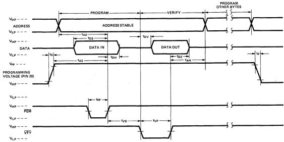
Figure 5. Programming Waveforms
