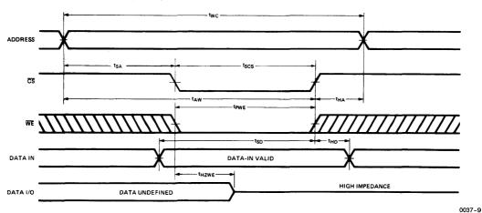
Note: If  $\overline{CS}$  goes high simultaneously with  $\overline{WE}$  high, the output remains in a high impedance state.
