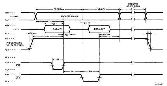
Figure 5. PROM Programming Waveforms
