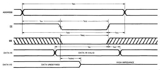
Note: If CE goes high simultaneously with WE high, the output remains in a high impedance state.
