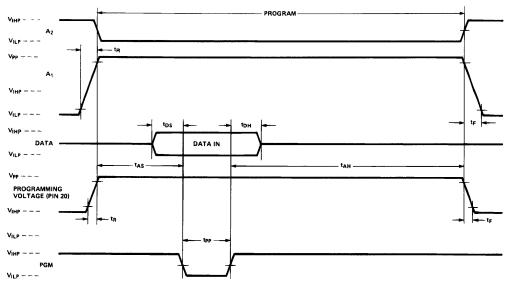
Figure 6. Initial Byte Programming Waveforms
