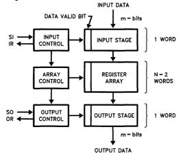
**Figure 1. Register Array Architecture**
