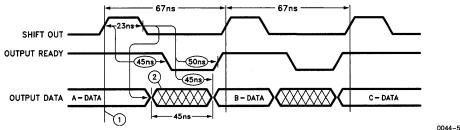
Figure 5. Output Timing for Register Array FIFO
