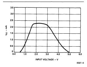
Figure 2. Input Voltage vs. Current
