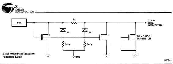
**Figure 4. Input Protection Circuit**
