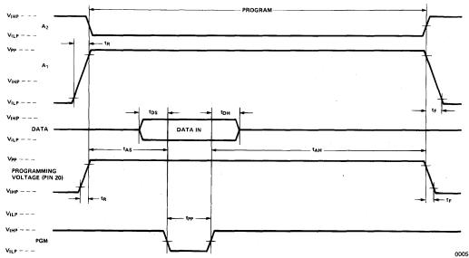
Figure 6. Initial Byte Programming Waveforms
