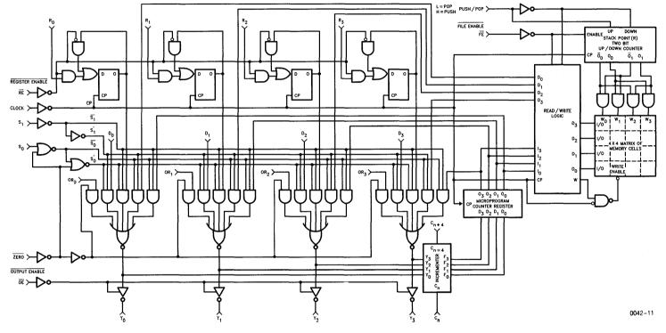
Figure 5. Microprogram Sequencer Block Diagram.
