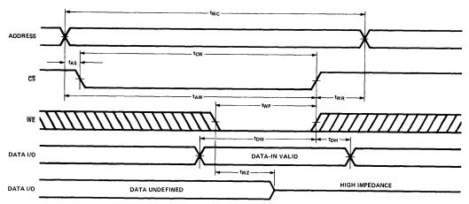
Note: If  $\overline{CS}$  goes high simultaneously with  $\overline{WE}$  high, the output remains in a high impedance state.
