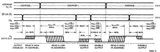
Switching delays from address input, output enable input and the chip select inputs to the data output. The CY93422 disabled output in the "OFF" condition is represented by a single center line.
