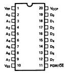
Figure 4. Programming Pin Configuration
