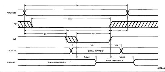
Write Cycle No. 2 (CS Controlled) (Note 7)
