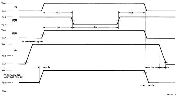
Figure 7. Program Synchronous Enable
