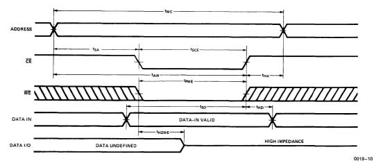
Note: If  $\overline{CE}$  goes high simultaneously with  $\overline{WE}$  high, the output remains in a high impedance state.
