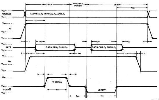
Figure 7. Program Waveforms Phantom Array
