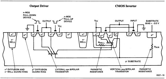
Figure 5. CMOS Cross Section and Parasitic Circuits
