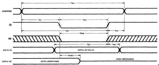
Note: If  $\overline{CE}$  goes high simultaneously with  $\overline{WE}$  high, the output remains in a high impedance state.
