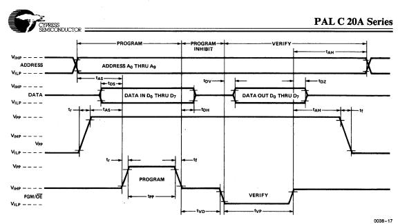
Figure 6. Programming Waveforms Normal Array
