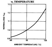
NORMALIZED SETUP TIME vs. TEMPERATURE
