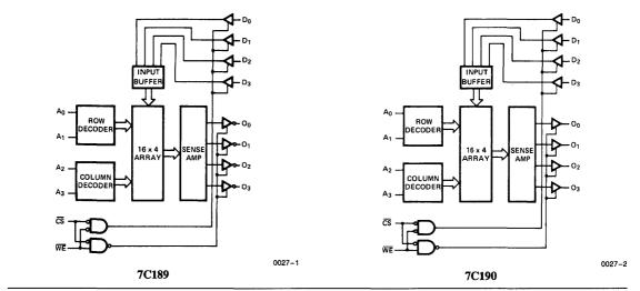
Figure 1. RAM Block Diagrams
