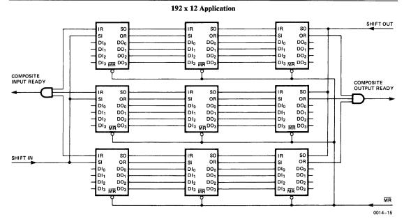
FIFOs are expandable in depth and width. However, in forming wider words two external gates are required to generate composite Input and Output Ready flags. This need is due to the variation of delays of the FIFOs.
