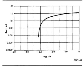
**Figure 7. Bias Generator Characteristics**
